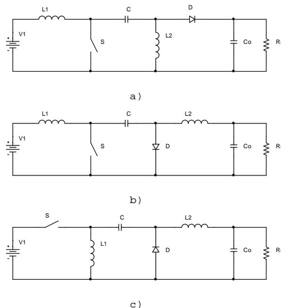
Figure 2. Developed DC-DC Converters: a) SEPIC converter, b) Cuk converter, c) ZETA converter
