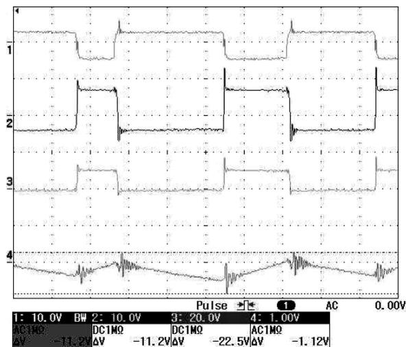
Figure 11. Waveforms of  $V_G$ ,  $V_D$ ,  $V_C$ ,  $\Delta V_o$  in conditions:  $V_1=7,1V$ ,  $V_o=3,4V$ ,  $R_S=5\Omega$
