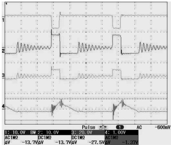
Figure 9. Waveforms of  $V_G$ ,  $V_D$ ,  $V_C$ ,  $\Delta V_o$  in conditions:  $V_i=8.3V$ ,  $V_o=3.3V$ ,  $R_s=20\Omega$
