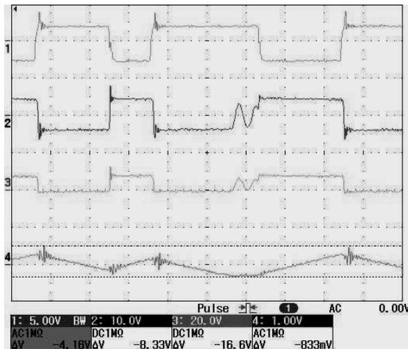
Figure 10. Waveforms of  $V_G$ ,  $V_D$ ,  $V_C$ ,  $\Delta V_o$  in conditions:  $V_i=4.9V$ ,  $V_o=3.4V$ ,  $R_s=10\Omega$
