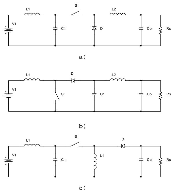
**Figure 1. Fundamental DC-DC Converters: a) buck converter, b) boost converter, c) buck-boost converter.**
