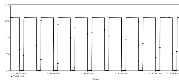
c)  $V_{stress}$  – voltage stress on switch
