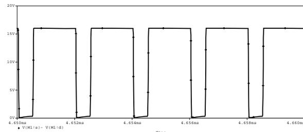
c)  $V_{stress}$  – voltage stress on switch
