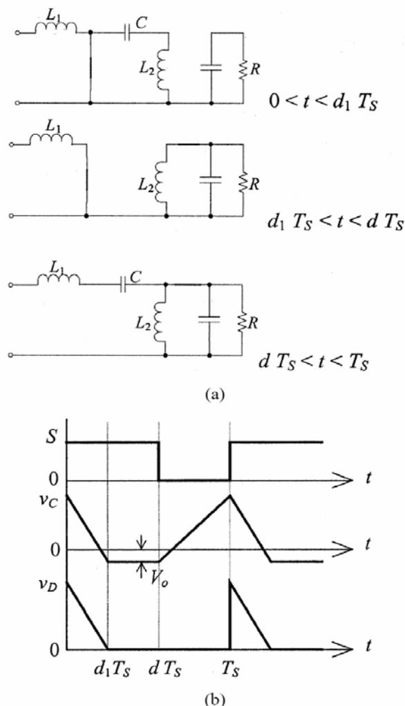
Figure 4. Operating principle of the SEPIC converter. a) equivalent circuits, b) theoretical waveforms [4]
