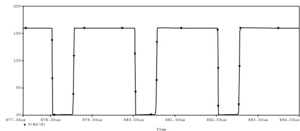
c)  $V_{stress}$  – voltage stress on switch
