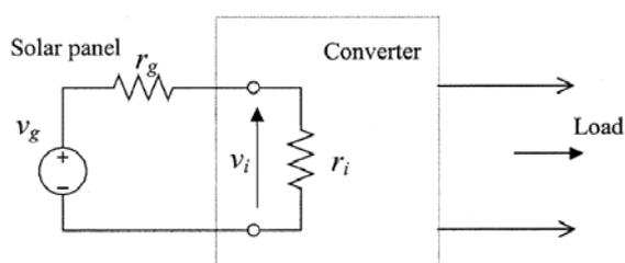
Figure 3. Equivalent circuit of a solar panel and converter [4]
