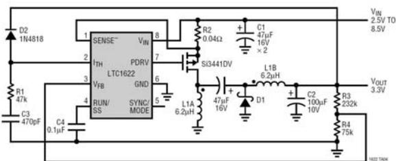
Figure 8. ZETA converter with LTC1622 [9]
